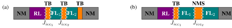
Figure 1: The intricate design of a multilayered MRAM cells in a more comprehensible form. (a) and (b) display a ultra-scaled MRAM cell. Color-coding is utilized for clear differentiation of components: the RL is marked in violet, the FL in teal, and the TB or NMS in orange. Non-magnetic (NM) contacts are represented in gray. Interfacial engineering regions are highlighted by white zigzag lines. The interaction strengths between the RL and the first FL ( FL_1 ) and between FL_1 and the second FL ( FL_2 ) are denoted by J_{iec_1} and J_{iec_2} , respectively.
