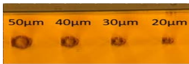
Fig. 1. End view of waveguides in Cr:ZnS crystal at \sim 200 \mu\text{m} depth (2090 nm writing). Laser beam is focused from above. Writing direction is perpendicular to the view plane. Since the index change in ZnS is negative, all waveguides are of depressed-cladding type, where the waveguide is formed by many lines of traces written around the unchanged core.
