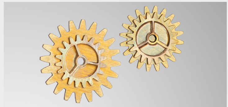
Cut and welded parts from brass using a single laser system.
